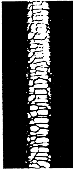
Fig. 2.11. Characteristic corn-cob structure of boron fiber. (From Ref. 15, used with permission.)
