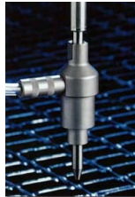
abrasive water jet up to 25 ft/min
