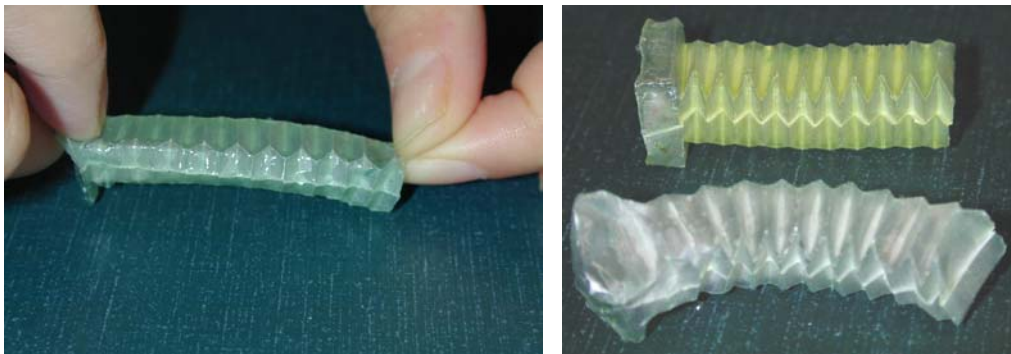
a) Hyper expansion of bellows b) Parylene bellows with(top) or without PDMS layer Fig 33. Comparison of Parylene bellows with or without PDMS
