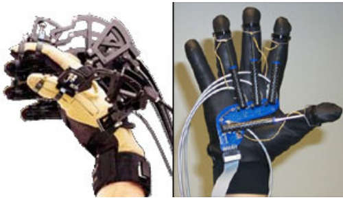
Fig. 2. The CyberGrasp [4] (left) and RM-II Hand Master [5] (right).
